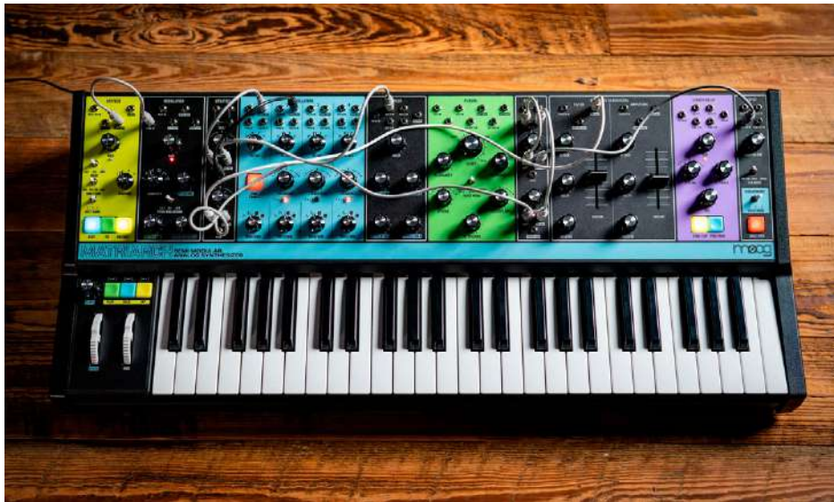
The analog stereo delay can also be used as a stand-alone effect device independent of the sound generation.
