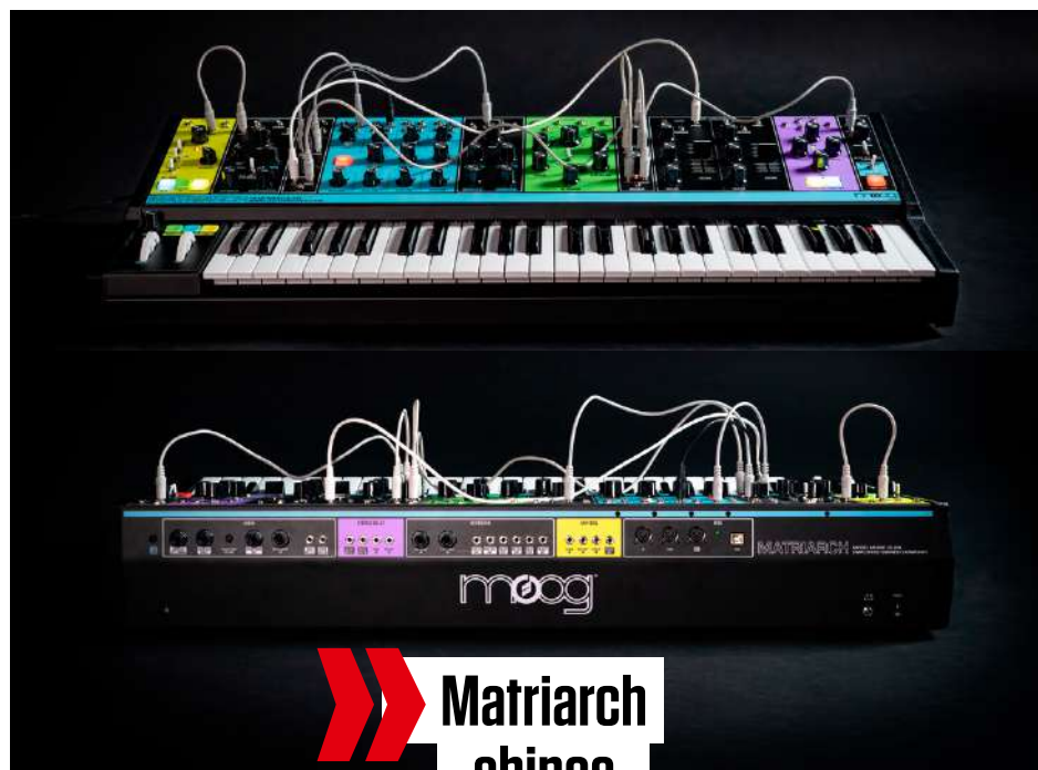
Matriarch consists of various modules that can be flexibly wired internally or connected to a modular system.
